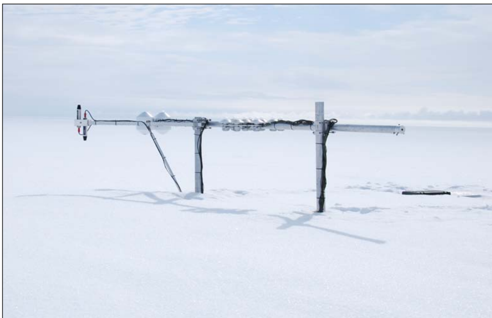
Figure 1: the radiation setup. From left to right: TriOS Ramses spectrometers; Kipp and Zonen pyranometers and pyrgeometers (CM21 and CG4, ventilated); Kipp and Zonen narrowband pyranometers (CM21, unventilated)
