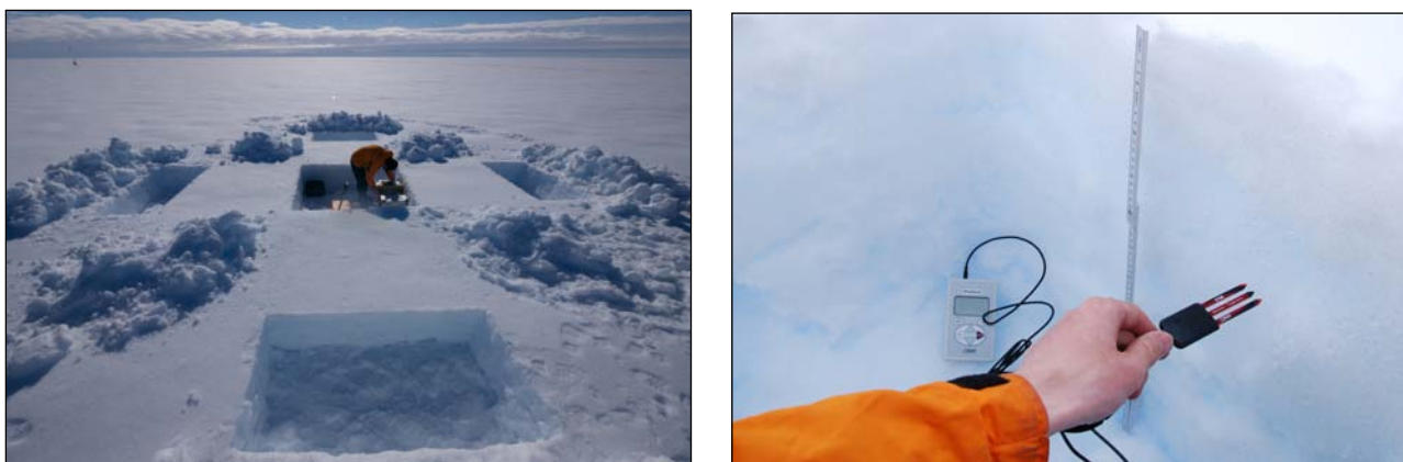
Figure 3: (left) Digging snow pits for inserting polyethylene tdr flatband cables. The datalogger is placed in the central pit, and the cables run from the central pit to each of the four outer pits. (right) Manual liquid water content measurements using Decagon 5TM probes and a Decagon ProCheck logger.
