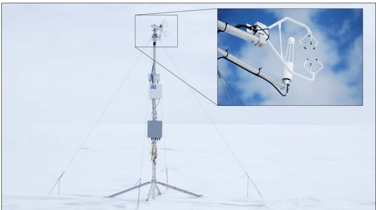
Figure 2: Turbulence mast with instruments at 4.0 metres above the snow surface. Dataloggers and instrument electronics are mounted on the vertical mast. The inset picture shows the Campbell CSAT3 sonic anemometer and the Li-Cor gas analyzer.
