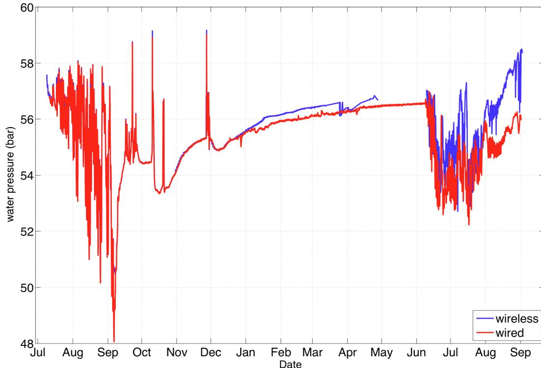
Figure 6. Subglacial pressure data from the wireless (blue) and wired (red) pressure sensors located in hole 1 and 2, respectively for the period July 2010 to September 2011.
