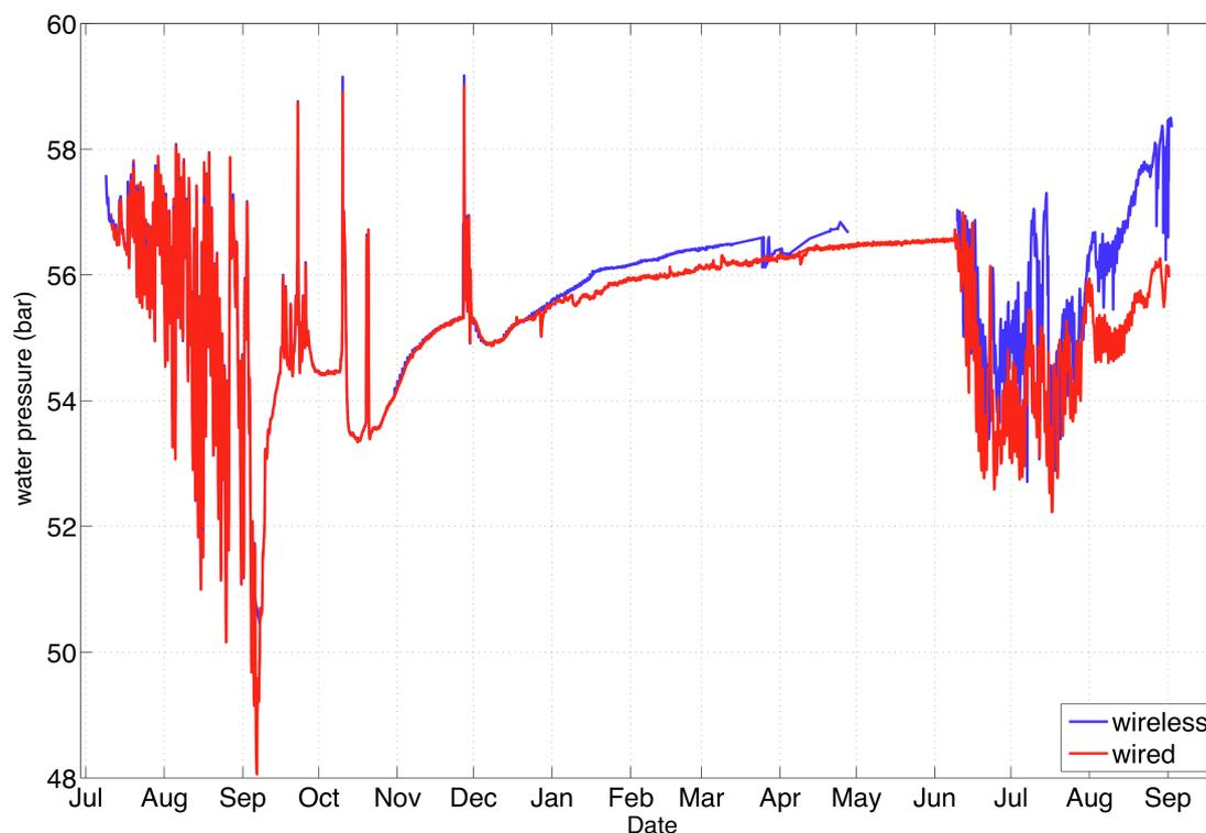
Figure 6. Subglacial pressure data from the wireless (blue) and wired (red) pressure sensors located in hole 1 and 2, respectively for the period July 2010 to September 2011.
