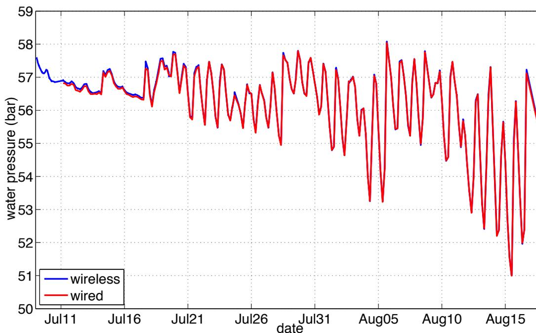
Figure 5. Subglacial pressure from the wireless (blue) and wired (red) pressure sensors located in hole 1 and 2, respectively during the period July 6<sup>th</sup> to August 18<sup>th</sup>, 2010.
