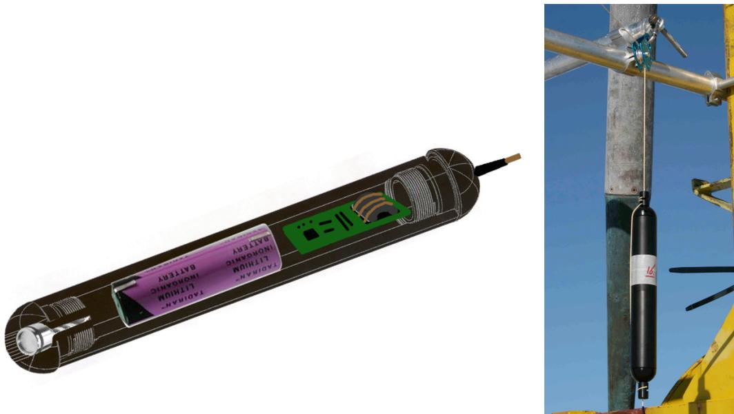
Figure 3. Left, an inside view of the probes used in the wireless subglacial measurement system. Right, probe number 16 attached to its Kevlar rope, ready to be lowered in hole 1. In the background the reamer drill head is visible.
