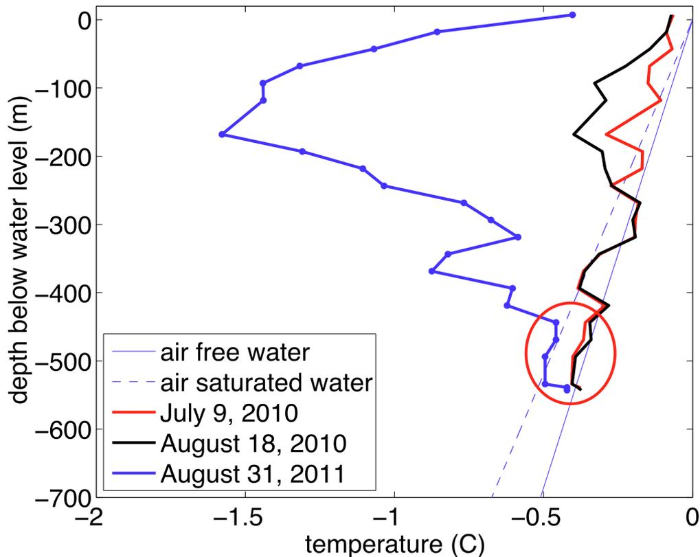
Figure 7. Average temperature profiles in hole 1 at July 9<sup>th</sup> (red) and August 18<sup>th</sup> (black) in 2010 and August 31<sup>st</sup> (blue) in 2011 as a function of depth below the water level, together with the theoretical curves for the melting point of air free and air saturated water (blue solid and dashed lines, respectively). The red circle indicates the lowest 7 temperature sensors and the pressure sensor.
