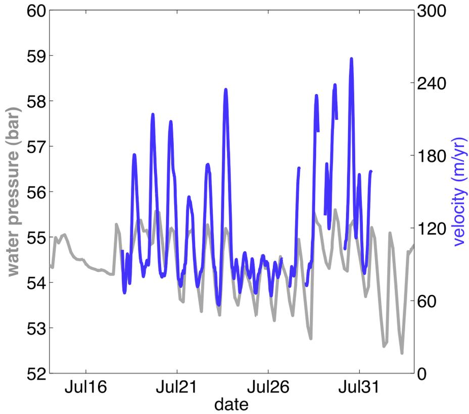
Figure 9. Subglacial water pressure and surface velocity from a geodetic GPS system near SHR for a period in July 2010.
