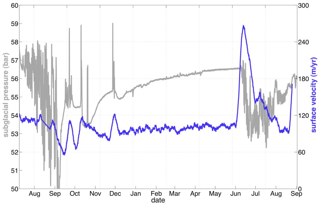
Figure 10. Subglacial water pressure and surface velocity (IMAU GPS system) for the period July 2010 to September 2011.
