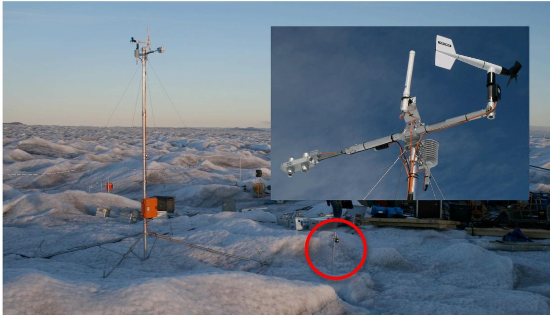
Figure 4. AWS at the drill site and a detailed view on the upper boom holding the sensors. The red circle indicates the sonic height ranger.
