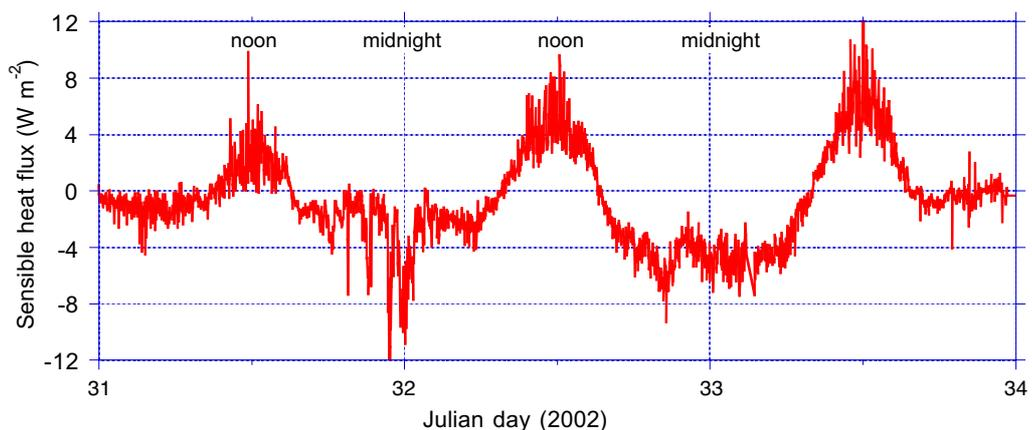
*Fig. 10. Sensible heat flux observed with sonic anemometer at 2 m, sampled at 20 Hz.*
