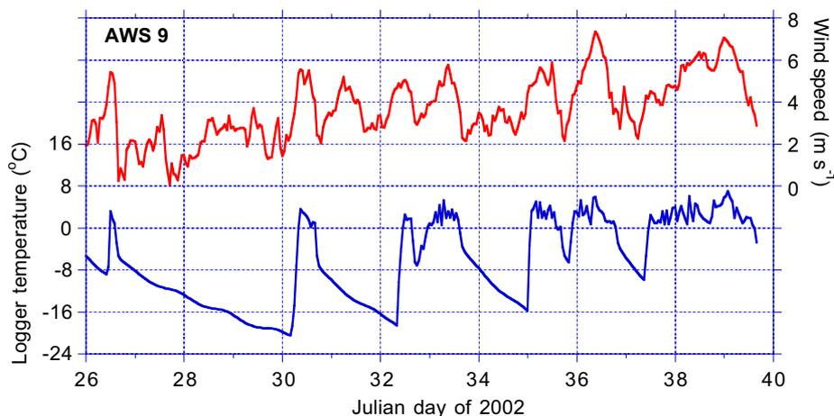
Fig. 13. Wind speed and logger temperature at AWS 9.
