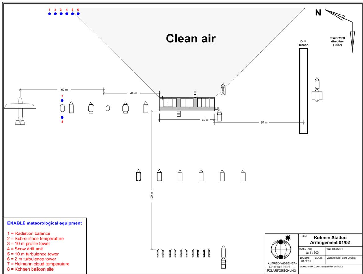
Fig. 4. Layout of Kohnen station and the various measurement sites of the meteorological experiment, highlighted in colour. Adapted from the original drawing by C. Drücker, AWI.
