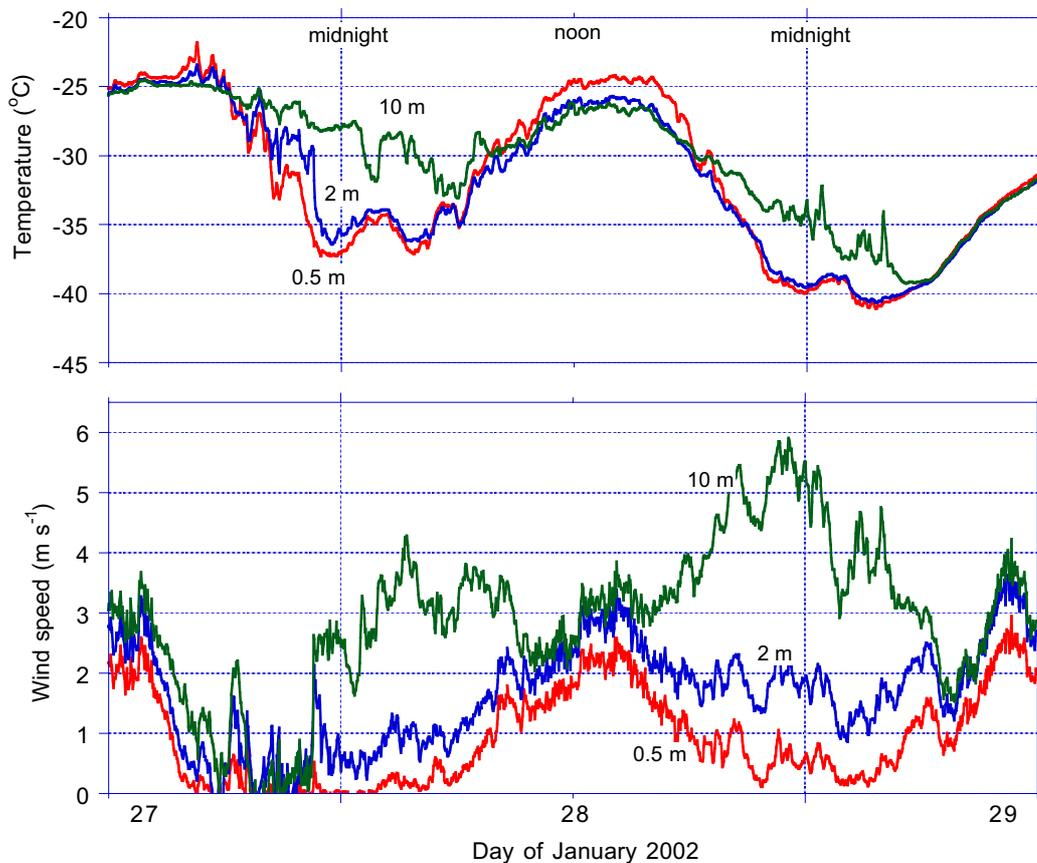
Fig. 6. Temperature and wind speed at 0.5 m, 2 m and 10 m (uncorrected) from the profile tower at Kohnen site, 27 to 29 January 2002.
