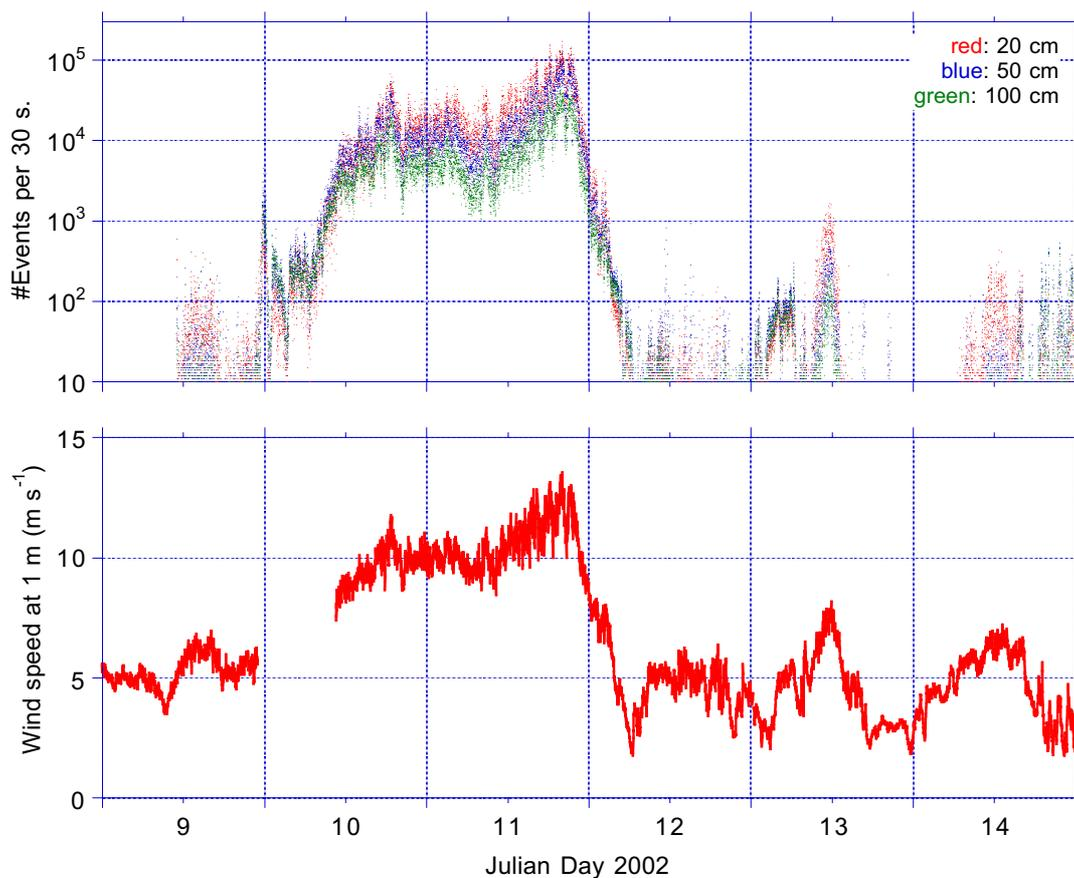
*Fig. 11. Number of particle impacts per 30 s at Kohnen at 20, 50 and 100 cm (upper panel) and 1 m wind speed (lower panel). Note logarithmic scale in upper panel.*
