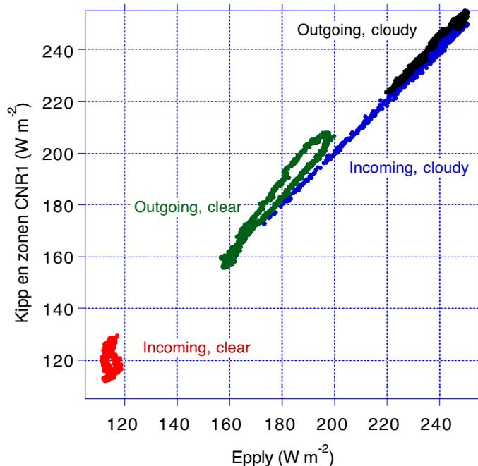
Fig. 7. Comparison of measured longwave radiation by two sensors (uncorrected data): Kipp en Zonen CNR1 (vertical axis) and Eppley PIR2 (horizontal axis), for a sunny day (January 31<sup>st</sup>) and a cloudy day (January 10<sup>th</sup>, 2002) during ENABLE.
