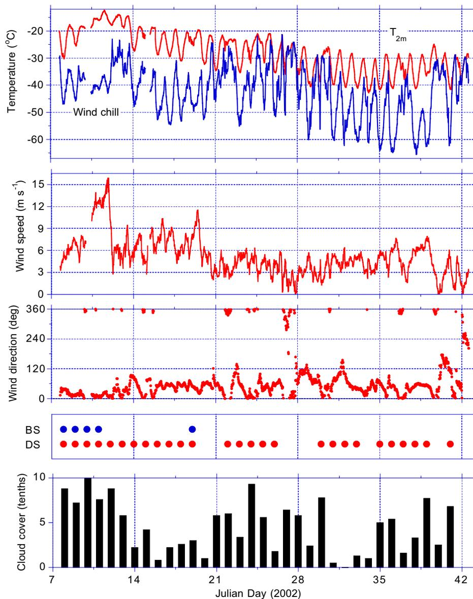
Fig. 5. Temperature at 2 m, wind chill, 10 m wind speed and direction, cloudiness and occurrence of drifting (DS) and/or blowing snow (BS) at Kohnen, 7 January to 10 February 2002.
