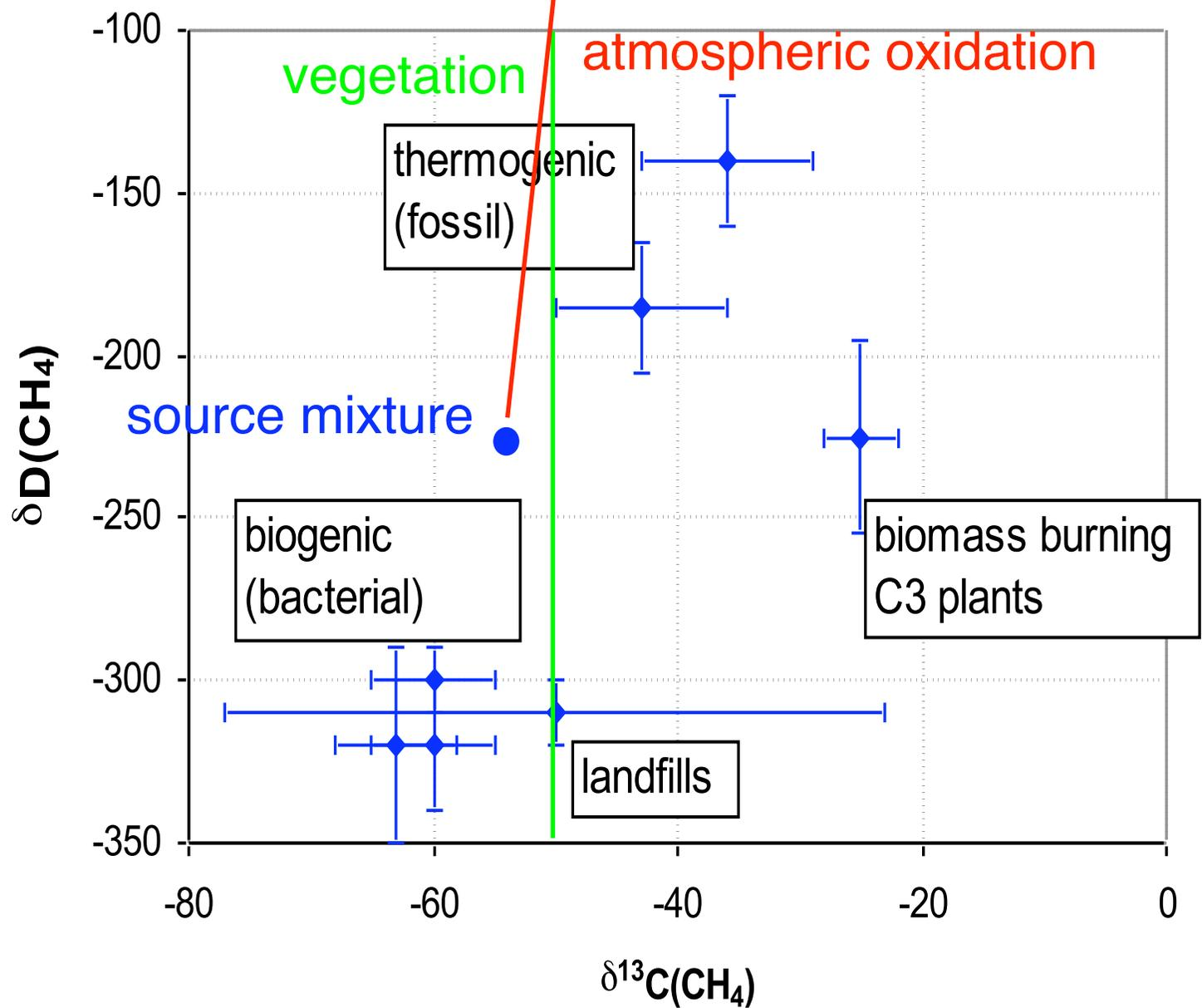
$$\delta^{13}\text{C} = \left[ \frac{^{13}\text{C}/^{12}\text{C}}{(^{13}\text{C}/^{12}\text{C})_{\text{ref}}} - 1 \right] \times 1000$$
