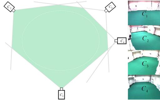
Figure 2. Top-view of the camera placement of the four monocular color cameras (*left*) and the camera views (*right*).
