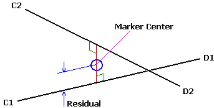
Figure 23 - Point residual determination with two cameras.
