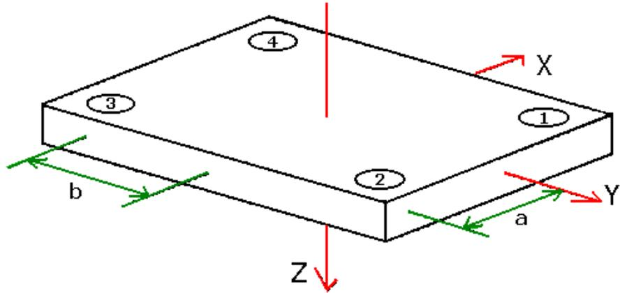
Figure 32 – ORIGIN data for eight channel force platforms.
