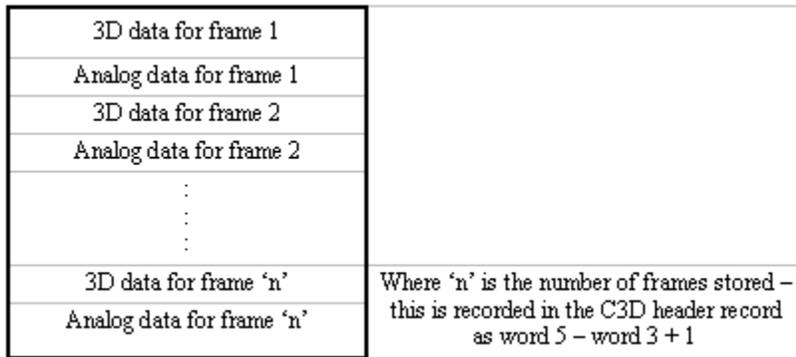
Figure 18 – The 3D / analog data storage structure.
