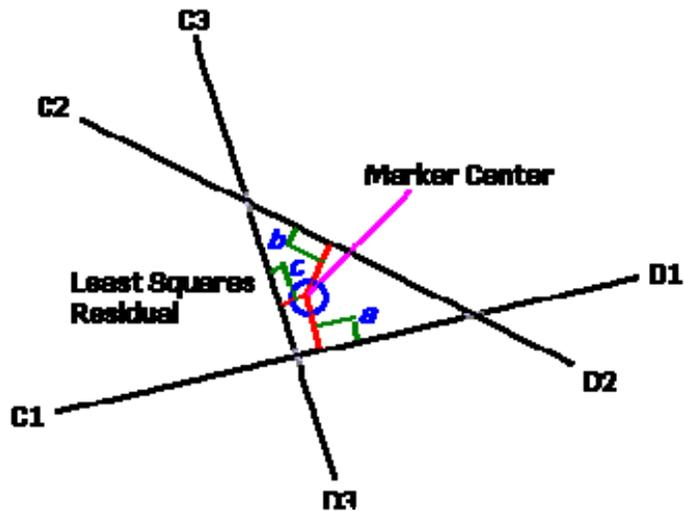
Figure 24 - Point residual determination with three cameras.
