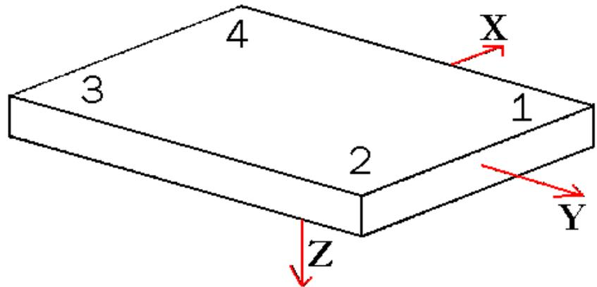
Figure 30 – The C3D force plate coordinate order.
